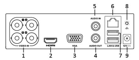
The rear panel of DS-7108HGHI-F1/N and DS-7116HGHI-F1/N provides 8 and 16 video input interfaces.
